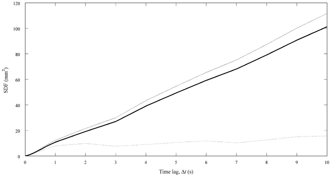
Fig. 5. SDFs of COP signals.  $\cdots$ , computed from  $u_{\text{ref}}$ ;  $\text{—}$ , computed from identified  $u_{\text{COP}}$ ;  $-\cdot-\cdot-$ , computed from  $u_{\text{COP}}$  with the initial set of parameters  $\mathbf{p} = \{K_p = 1117.27 \text{ N m rad}^{-1}, K_I = 14.32 \text{ N m rad}^{-1} \text{ s}^{-1}, K_D = 257.83 \text{ N m rad}^{-1} \text{ s}\}$ .
