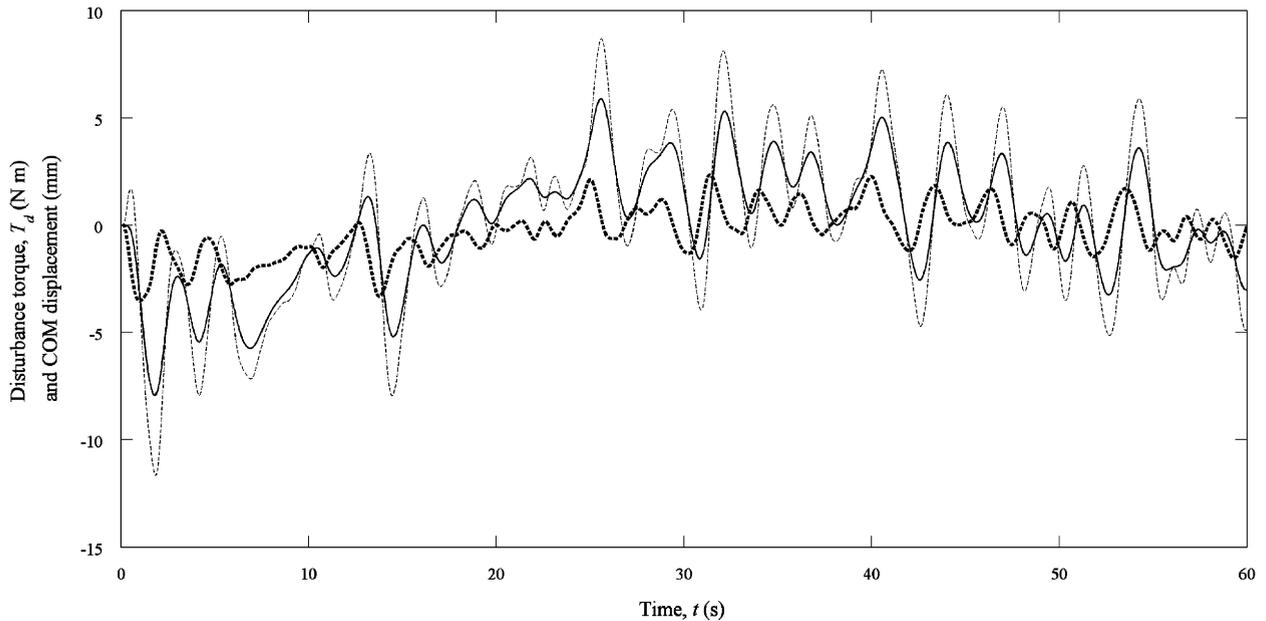
Fig. 7. Comparison of signal shapes. . . . ., disturbance torque  $T_d$ ; ---, COM signal produced by CIP model with “center normal” parameters set  $\mathbf{p}$ ; —, COM signal produced by CIP model with identified (right column of Table 2) parameters set  $\mathbf{p}$ .
